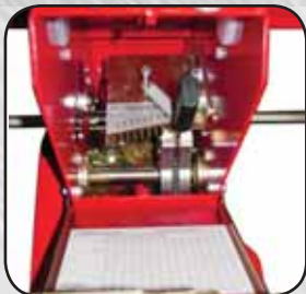
Easy to change seed spacing with shifttable 10 speed transmission
