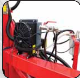
Special air cooling fan removes moisture from the seeding system
