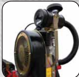
Separate air compressor system cleans out each seed hole after seed is deposited
