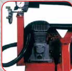
Separate air compressor system cleans out each seed hole after seed is deposited
