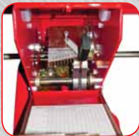
Easy to change seed spacing with shiftable 10 speed transmission
