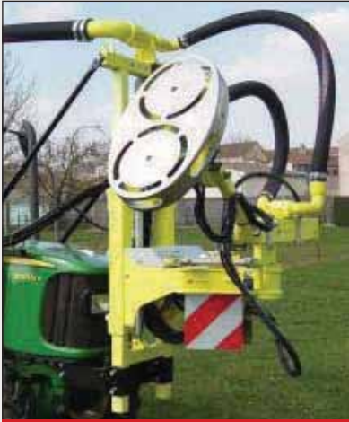
Elliptical shaped dual rotor defoliation head
