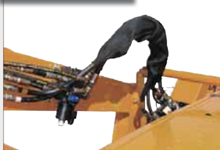
Model # EH-100 Electro Hydraulic Valve components for installation on tractor loaders
