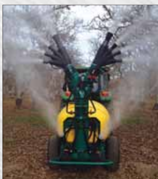
The cannon Venturi Air Sprayer operating in 45 foot high walnut orchard at 50 gallons per acre.
