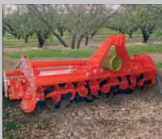
S Tiller with Adjustable Rear Roller
