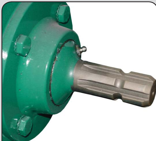
Built-in overrunning clutch to protect drive train
