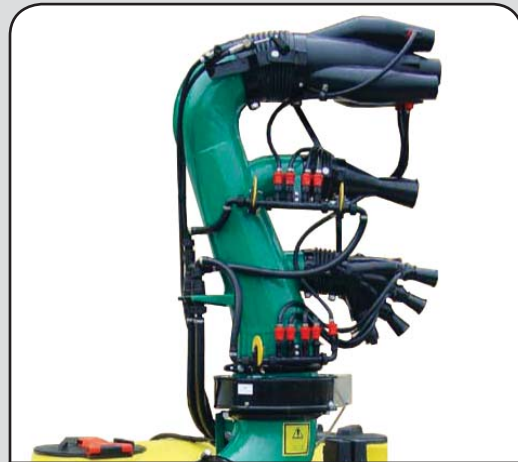
14 Different heads available, horizontal cannons that spray up to 90' shown
