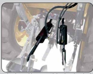
To make box scrapers more versatile, nothing works better than being able to control the tilt and pitch of the implement. Grading jobs are more accurate because you have complete control to develop the slopes you require when landscaping, building roads, etc.
