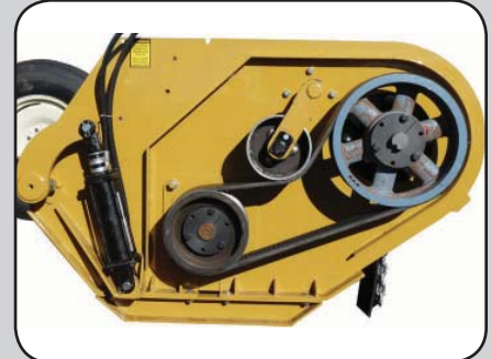
6 Belt drive with 8 1/2" spring loaded idler & optional cylinders
