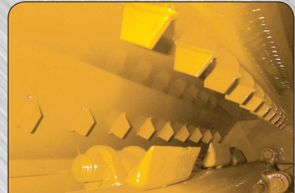
Rotor shaft, hammer knives and re-cutter blades
