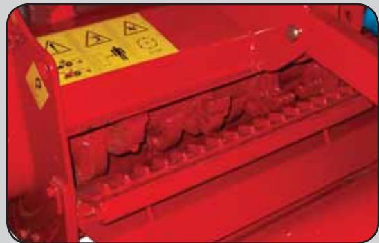
Two access doors to the steel plate screen interior
