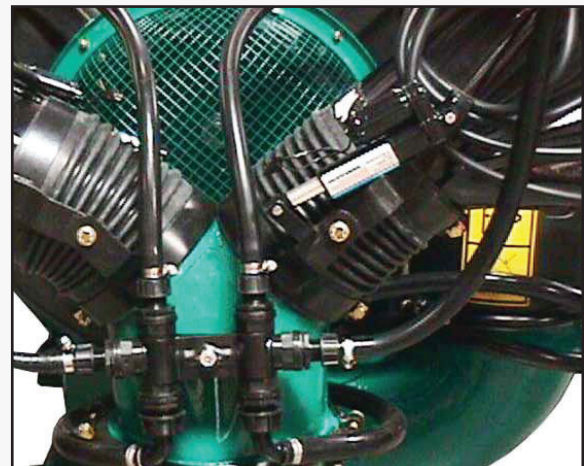
Optional Electro Cylinders To Adjust Nozzles For Different Plant Heights
