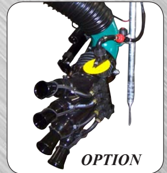
Electro cylinders with control box operated from tractor seat (outer spray heads)
