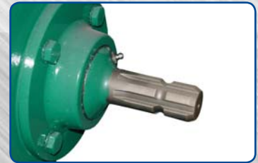
Built-in overrunning clutch to protect drive train
