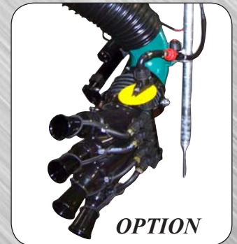
Electro cylinders with control box operated from tractor seat (outer spray heads)
