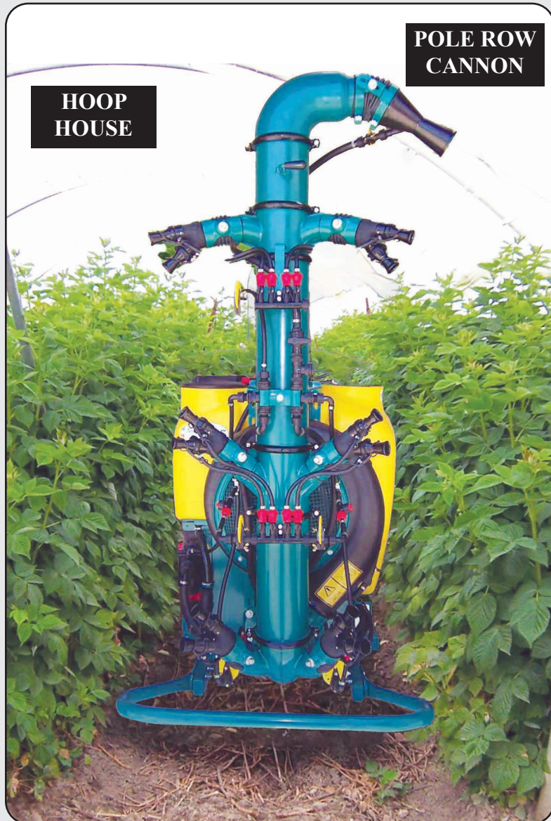
Hoop Houses - Spray with the 12 Venturi nozzle distribution head in the open rows.
