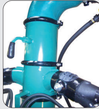
Shutter Extension with air shut off handle
