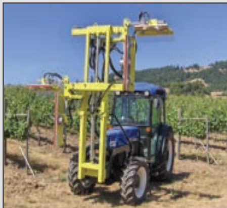
Model P2200TS Trims 2 Half Rows, Terraced Vineyard
