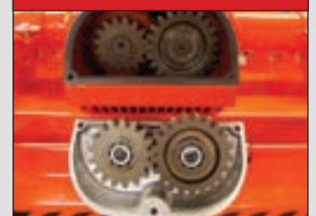
Quick change speeds on 4 Speed Gearbox
