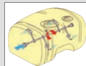
Centrifugal pump powers rotating liquid agitation system to insure product mix
