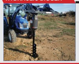
The D450 hydraulic digger is the most trouble free digger on the market. The unit features an in line sealed planetary gear reduction drive design. This clean, effective system ensures long trouble free usage. Digger comes with Q.A. brackets w/cradle.
