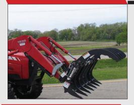
The aggressive tine shanks root out objects below ground level. The wide grapple opening allows for gathering a large amount of brush and debris. The hydraulically operated grapple locks the material in place and stabilizes it for transport.
